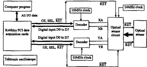
Figure 6 Schematics showing signal processing of the sensor
