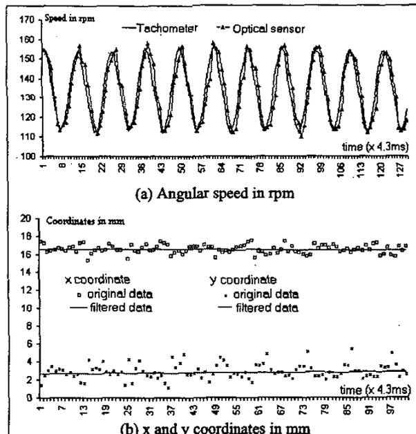
Figure 14: 3-DOF Sensor response to sinusoidal input
