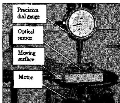
Figure 11 Test of sensor-surface spacing
