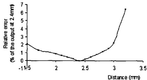
Figure 12 Effects of sensor-surface spacing
