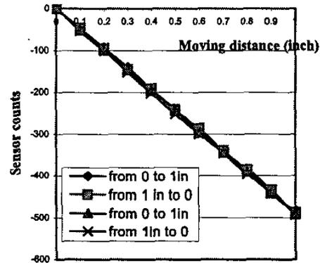
Figure 9 Test results of sensor repeatability ( $C_r=495\text{cpi}$ )
