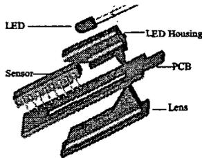
Figure 4 Exploded view of an optical sensor
