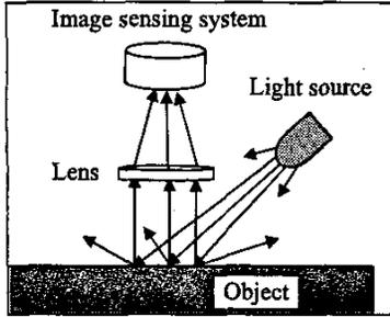
Figure 1: A typical imaging system
