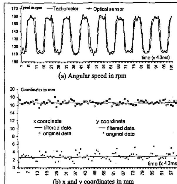
Figure 15: 3-DOF Sensor response to sinusoidal input
