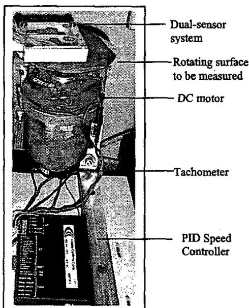
Figure 10 Experimental setup of a dual-sensor system
