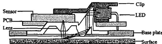
Figure 5 Assembly view illustrating the principle
